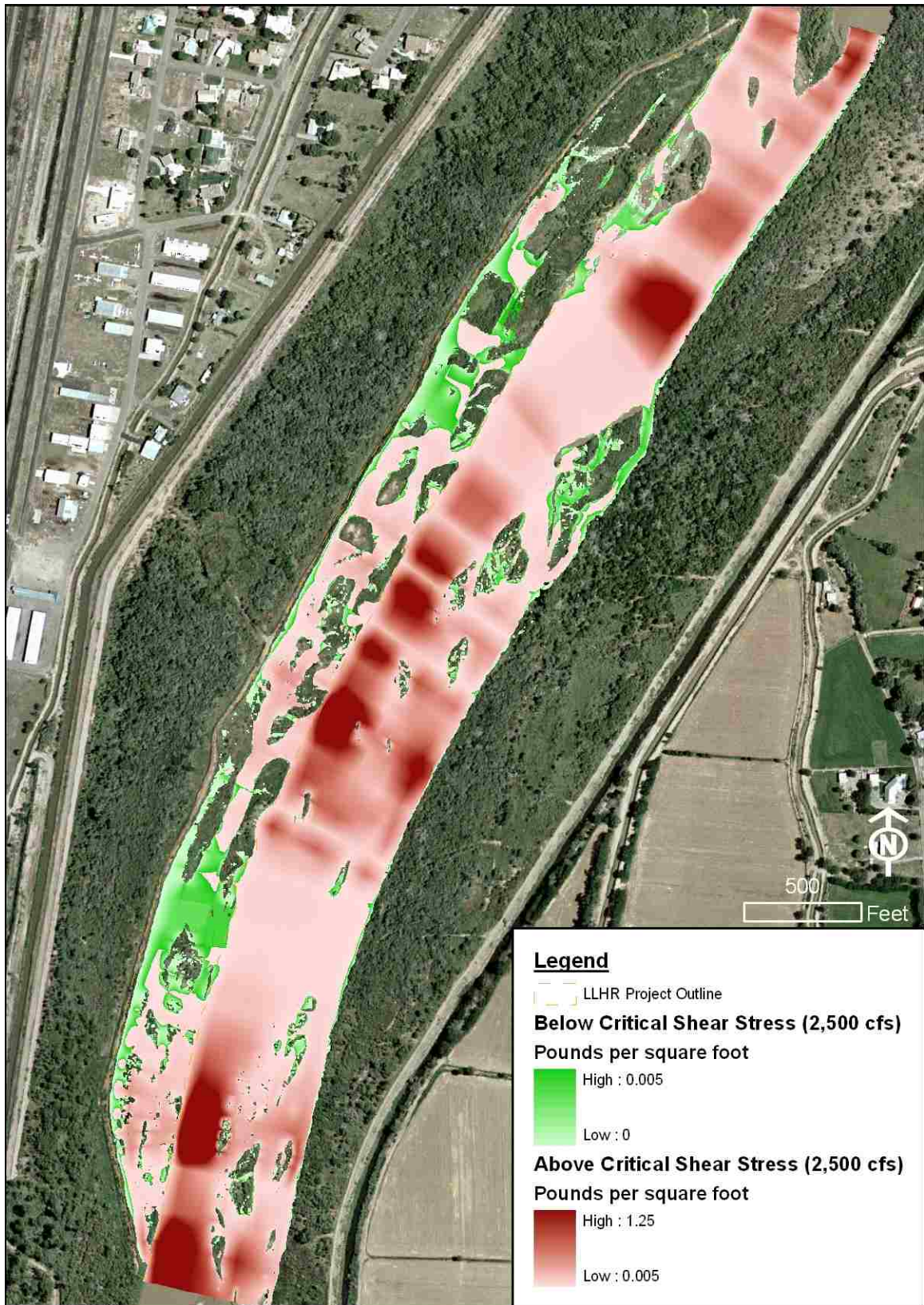
Figure 21: Shear stress map for the 2,500 cfs flow regime
