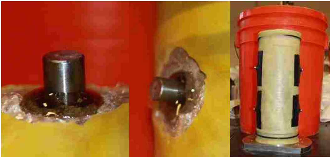
Figure 3.17 Epoxied Button Examples
