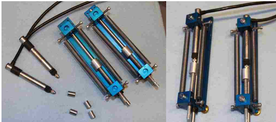
Figure 3.16 LVDT Setup for Glued Button Deformation Measurement
