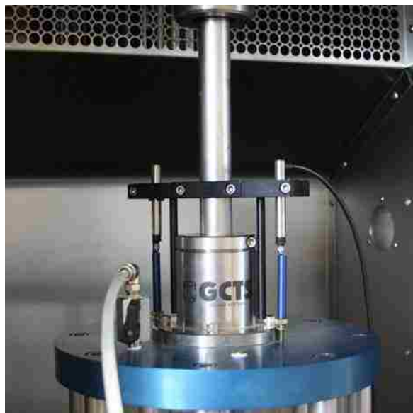
Figure 3.19 External LVDT Setup Clamped to Loading Piston
