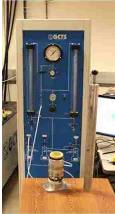
Figure 3.9 Mold Setup with Membrane and Applied Vacuum
