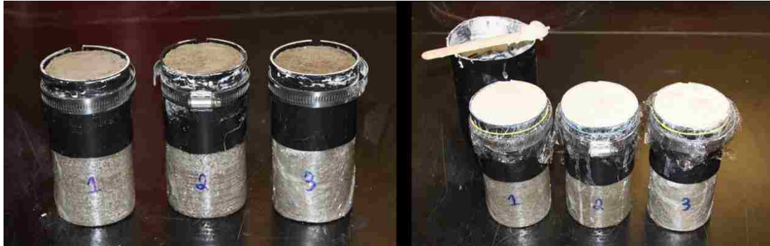
Figure 3.10 Example of Gypsum Cement Capping Method
