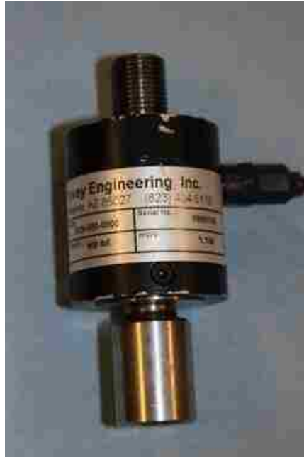
Figure 3.12 Load Cell for Used For Resilient Modulus and Alternate Testing
