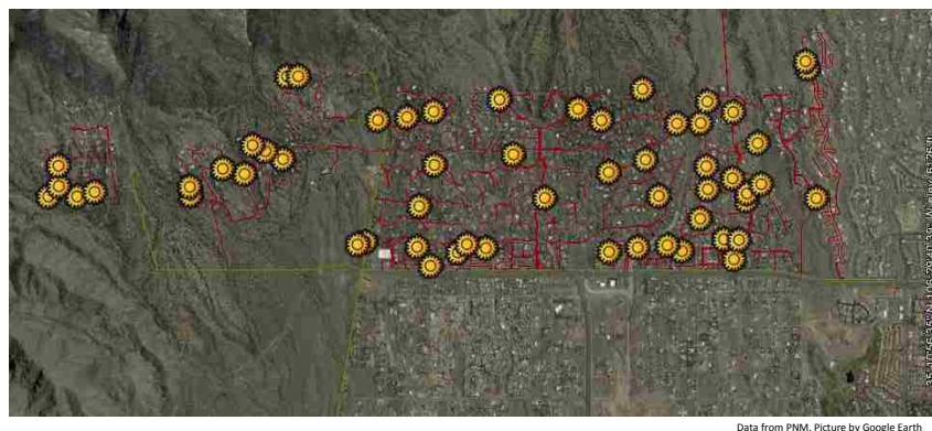
Figure 3.3: Top-view outline of Tramway11 feeder in 2012 by Google Earth. Installed rooftop PV systems are illustrated.
