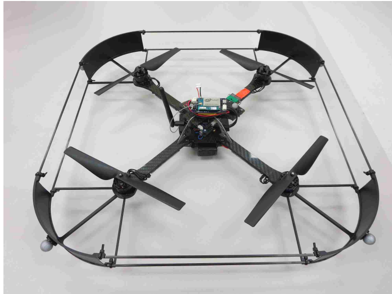
Figure 2.3: AscTec Hummingbird quadrotor with a large protection frame, Intel Edison control board, and Wi-Fi antenna. The orange tape indicates the “front” quadrotor arm.
