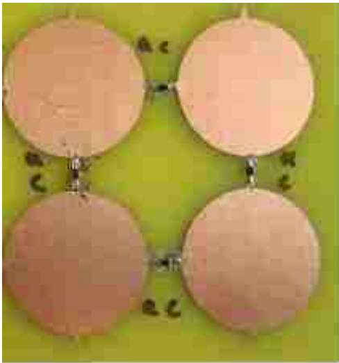
Figure 14: 2x2 Circular dipole rectenna array operating from 2.4 GHz to 6.6 GHz with a rectified voltage of 75 mV [7].
