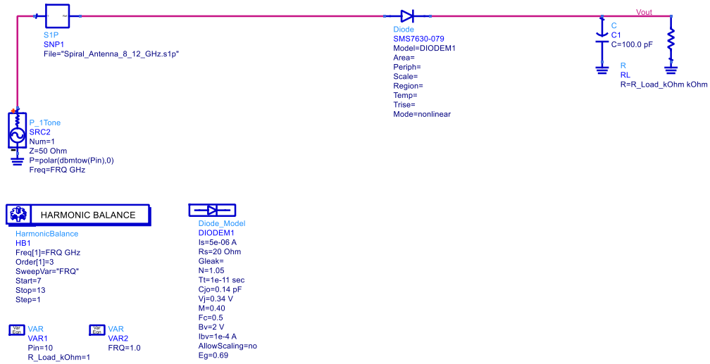
Figure 106: ADS Circuit for Spiral Rectenna with 10 dBm input power and a 1 kOhm load.
