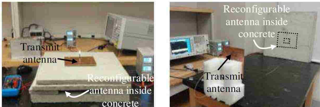
Figure 25: Example of the Reconfigurable stacked patch communication rectenna performing rectification and data communication in a concrete slab with a rectified voltage of 2.1 Volts [12].
