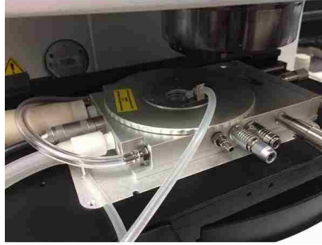
Figure 2.5: Absolute absorption measurement of a photodetector with an infrared microscope
