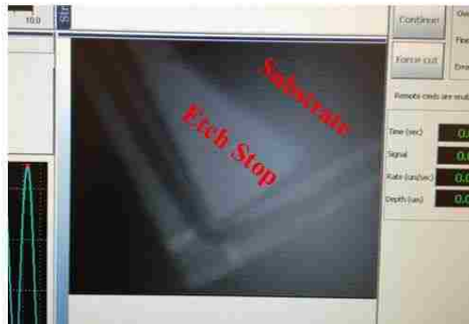
Figure 4.11: Corner image of an FPA during substrate removal with the AlAsSb etch stop partially exposed
