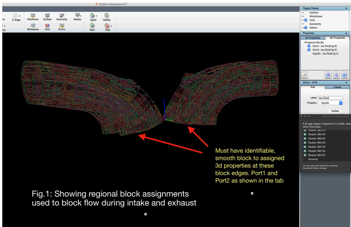
Figure B.4: Schematic breakdown of the FEARCE/GridPro moving marker valve overlay 3D port blocking properties.
