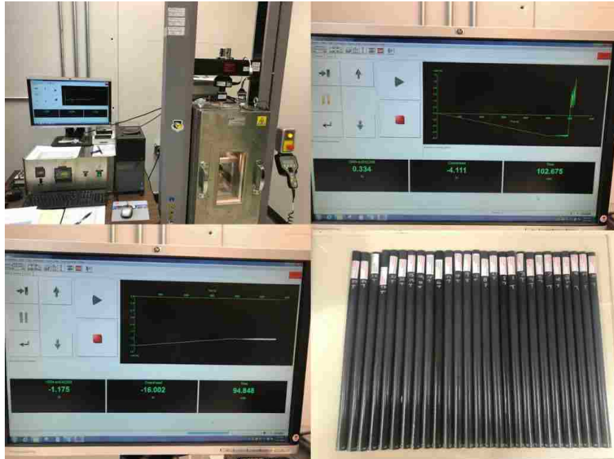
Figure 3.25 Full Test Setup and 26 Control Tape Springs Post Structural Testing
