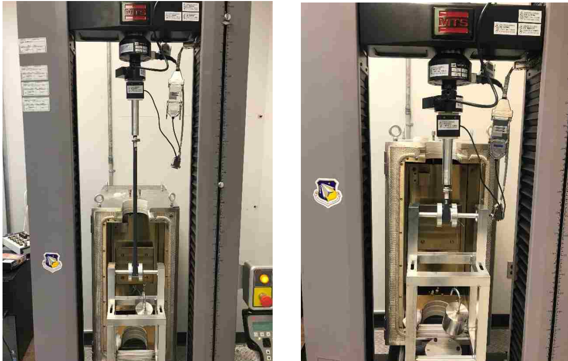
Figure 3.31 ANP Tape Spring Structural Testing One Hour and One Day
