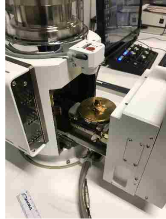
Figure 3.34 JEOL-JSM-IT100 SEM/EDS for ANP Dispersion Examination
