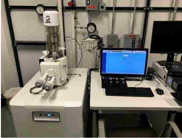
Figure 3.34 JEOL-JSM-IT100 SEM/EDS for ANP Dispersion Examination
