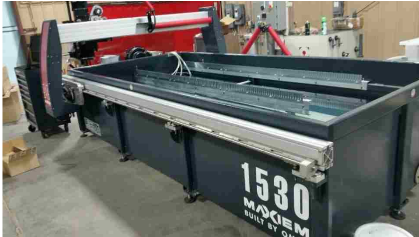
Figure 3.10 Waterjet Cutting Machine at Holloman Air Force Base
