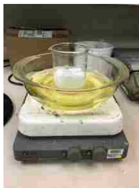
Figure 3.4 Preparation of Neat Epoxy
