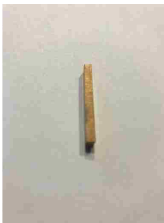
Figure 3.43 Gold-Sputtered ANP Epoxy Coupon
