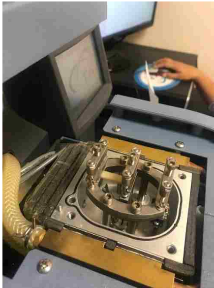
Figure 3.27 DMA Testing of ANP Coupons
