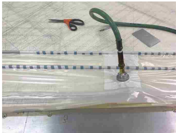
Figure 3.29 Vacuum Bagging Process for Fabrication of Tape Springs
