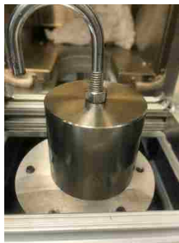
Figure 3.20 Counter Mass for Tape Springs’ Structural Testing
