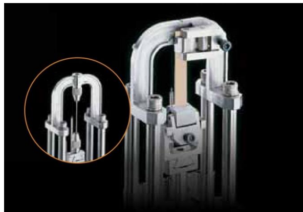
Figure 37: Tension clamp experimental setup 48
