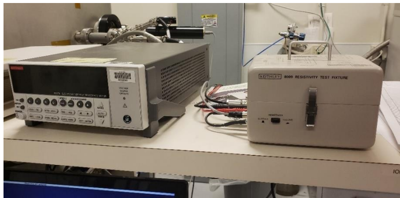
Figure 22: Electrical conductivity measurement test setup
