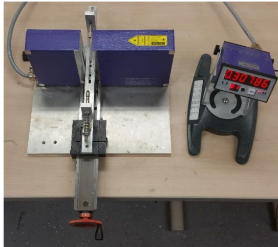
Figure 4-1: Laser micrometer setup with custom-made sample holder for measuring the diameter of Nylon and Copper wire substrates as well as CNT coated composite wires
