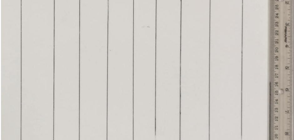
Figure 3-4: CNT coated samples with nylon core
