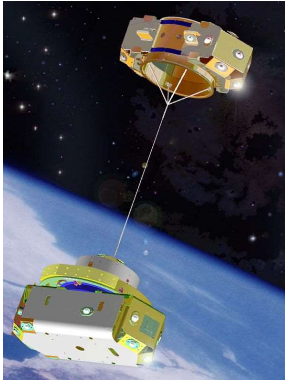
Figure 1. Artist Portrayal of NRL's TiPS in Deployed Configuration
