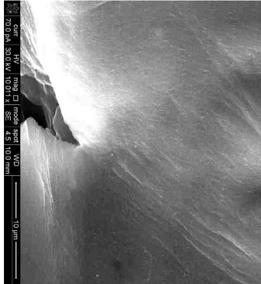
Figure 48 Zoomed in SEM picture of the red box shown in figure 47. This picture is showing us the tip of the void that is being created by the tension. Here we can see that the void is spreading in the direction of the shear banding which will ultimately cas the part to fracture.
