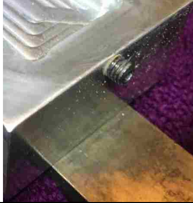
Figure 7 This image is showing a small set screw that was on one end of the holder that was used to pinch the sample into the holder. This was to prevent the sample from having any movement during the sanding and polishing process.
