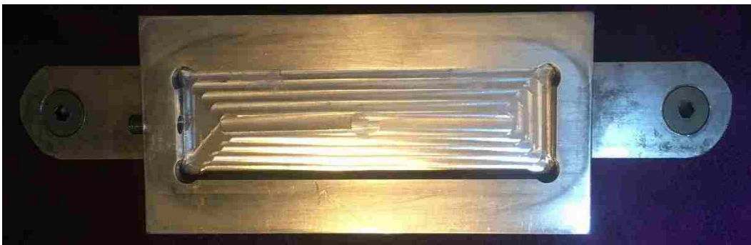
Figure 6 This is the bottom view of the holder showing where the sample will be held. The depth of the slot used to hold the sample was slightly less than the overall thickness of the samples.
