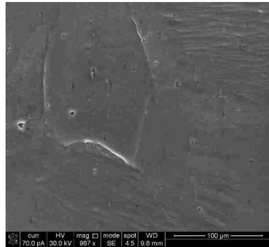
Figure 42 Zoomed in SEM picture of the yellow box in figure 40 at 1000x magnification. In this picture we can clearly see the outer boundaries of a grain that is resisting the dislocations in the material.
