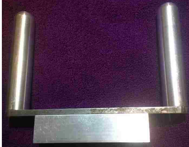
Figure 5 This is a picture of the holder that was created to hold the samples while they were being sanded and polished. The handles were spread out evenly so that an even amount of pressure can be applied to make the samples as flat as possible.
