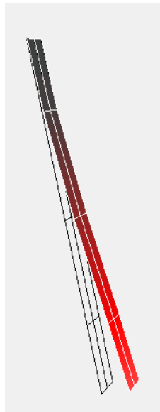
Figure 12: First Bending Mode from 1D LDV
