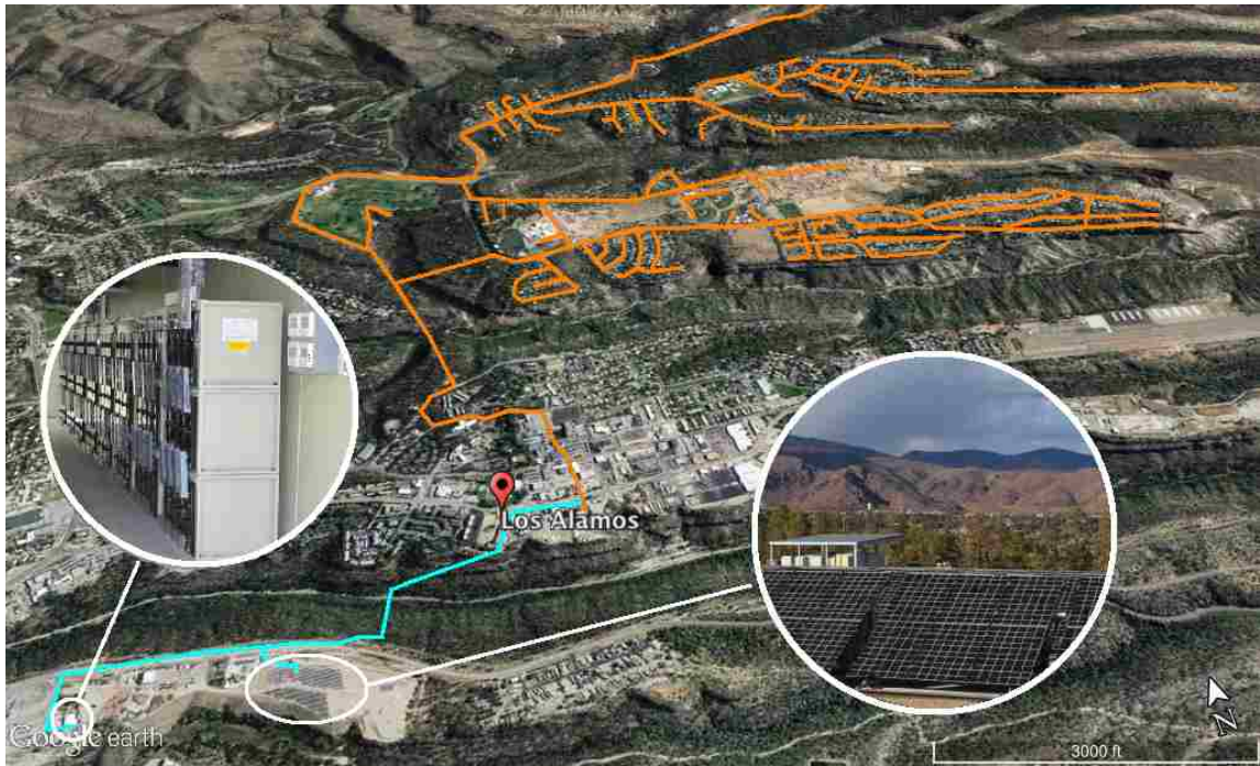
Fig. 1: The Circuit 16 feeder, outlined in orange, serves the Northeast area of Los Alamos, NM, covering mainly the Barranca and North Mesas. The battery storage and PV array are located at the local landfill and they interconnect to Circuit 16 at the substation, outlined in blue. Customers served by Circuit 16 include a 1600-home smart community, apartment complex, middle & elementary schools, a sports complex, a golf course, water distribution infrastructure, among others.
