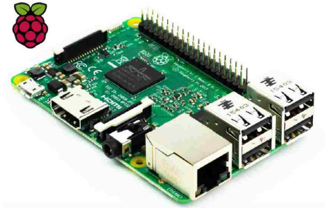
Fig. 15: Raspberry Pi 3, credit-card-sized single board computers running Linux operating systems.
