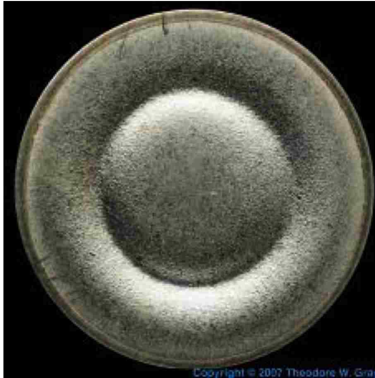
Figure 2.2 Sputtering target showing characteristic erosion pattern
