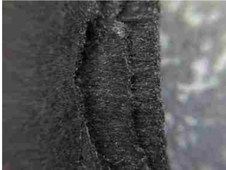
Figure 31 Fracture surface of carbon fiber composite specimen
