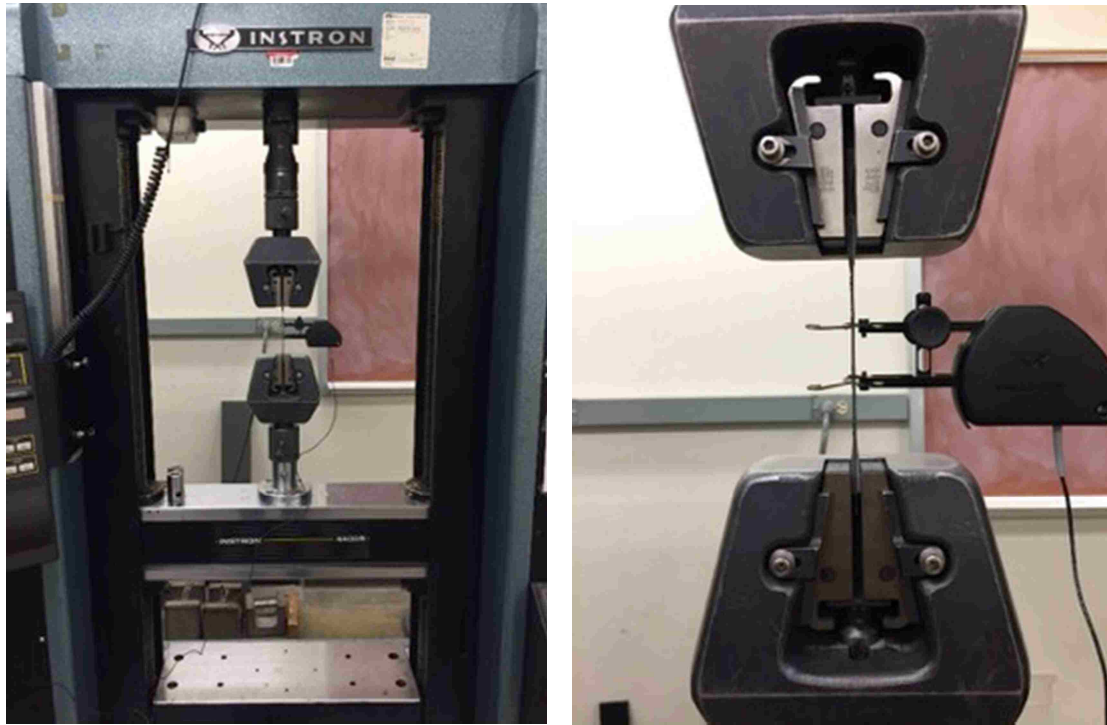
Figure 35 Instron 4400R tensile test setup. The extensometer is attached with rectangular clips.
