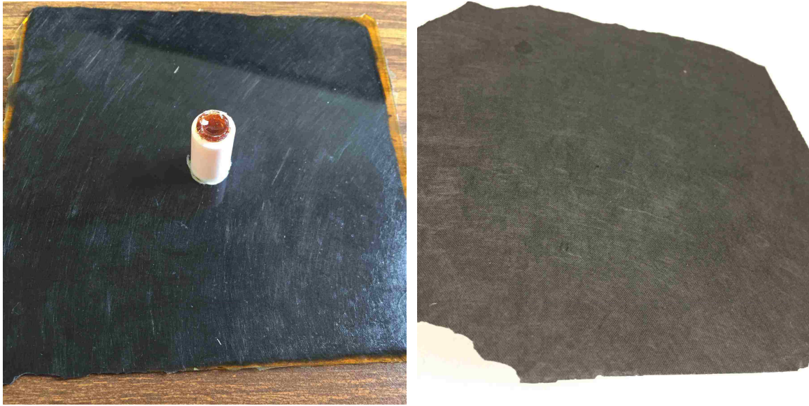
Figure 28 Examples of rCF composites manufactured using RTM (left) and wet-layup (right)
