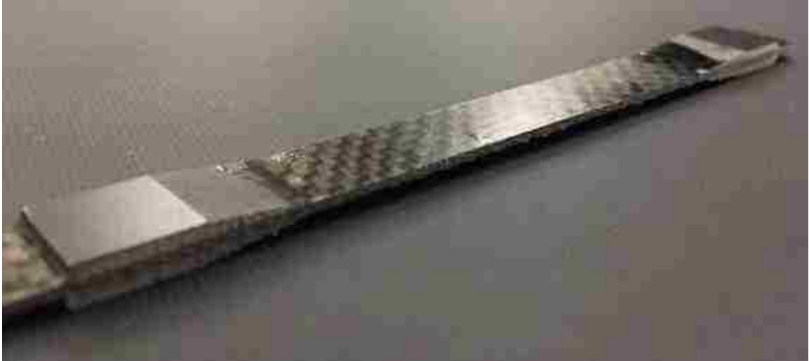
Figure 34 Example of tensile coupon and tab geometry.
