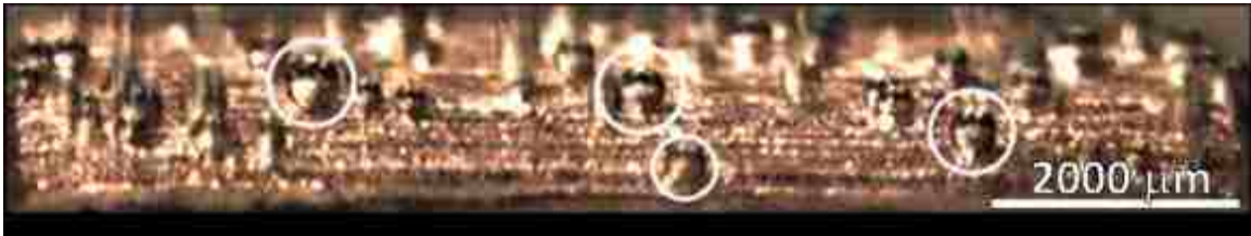
Figure 3.8. An example of a single captured frame of the full boiling surface used to identify discrete bubble locations in saturated boiling of PF-5060 dielectric liquid.
