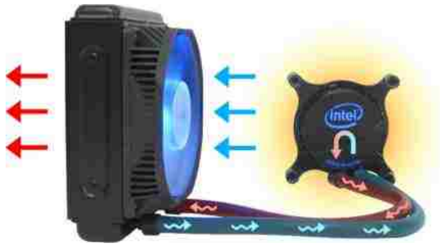
Figure 2.2. The closed loop liquid cooler is a high performance microprocessor cooling alternative to high end air cooling.
