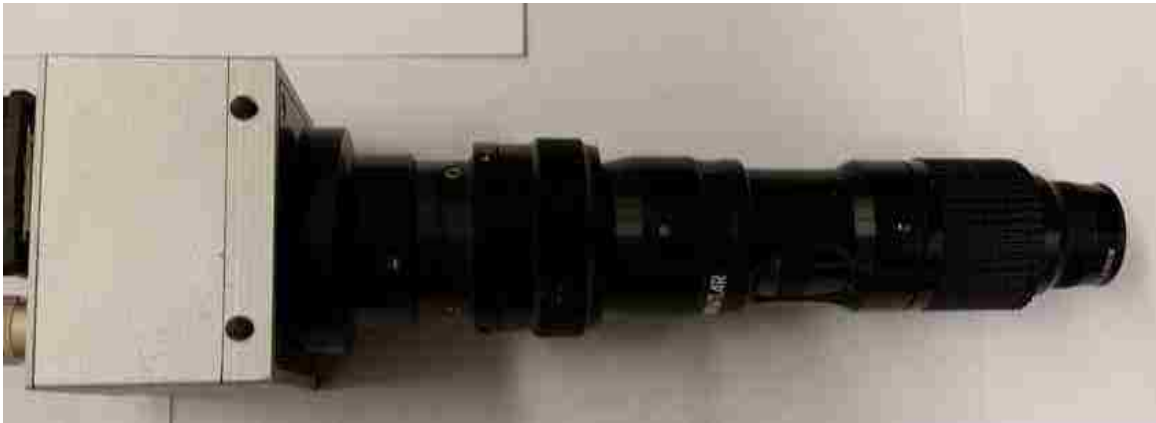
Figure 3.7. The high-speed video camera used to capture images of individual bubble transient growths at 210 fps.
