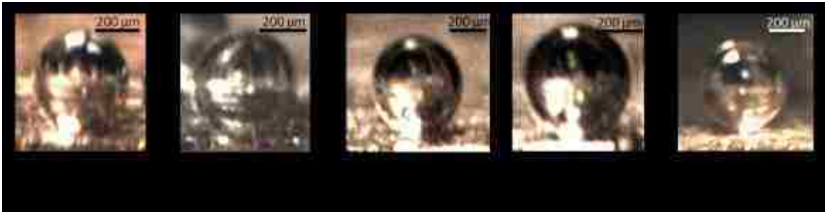
Figure 4.32 Captured images of discrete bubbles on various surfaces just before departure.
