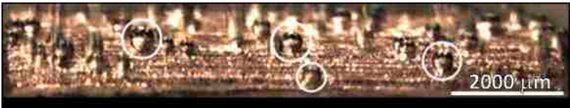
Figure 4.31 A single frame of the full boiling surface with R_a = 1.44 \mu\text{m} used to identify discrete bubble locations.
