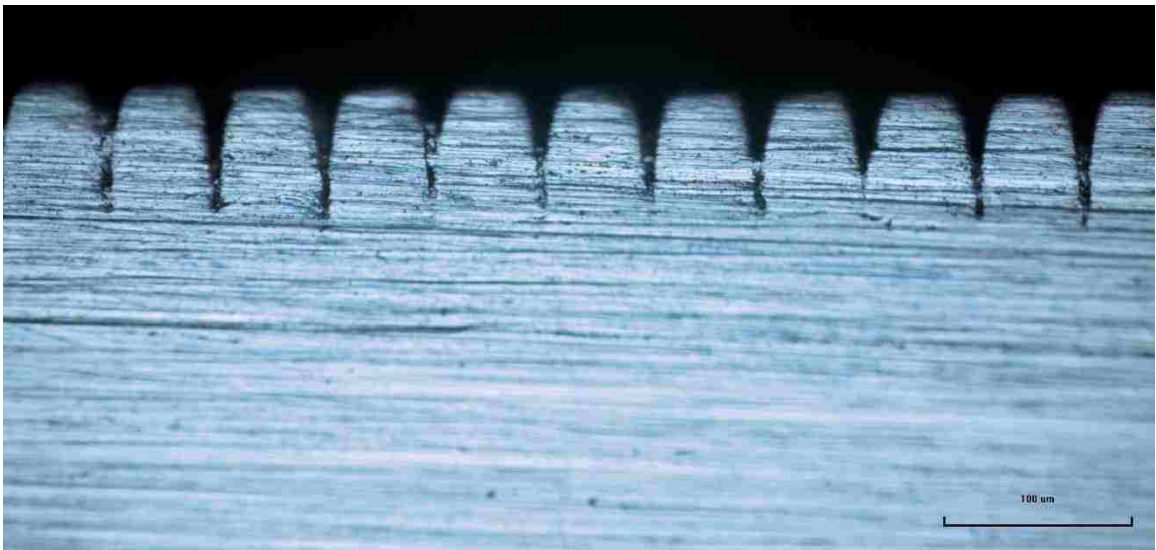
Figure 5-4: Side view microscope image of laser machined microchannels at 20x magnification.
