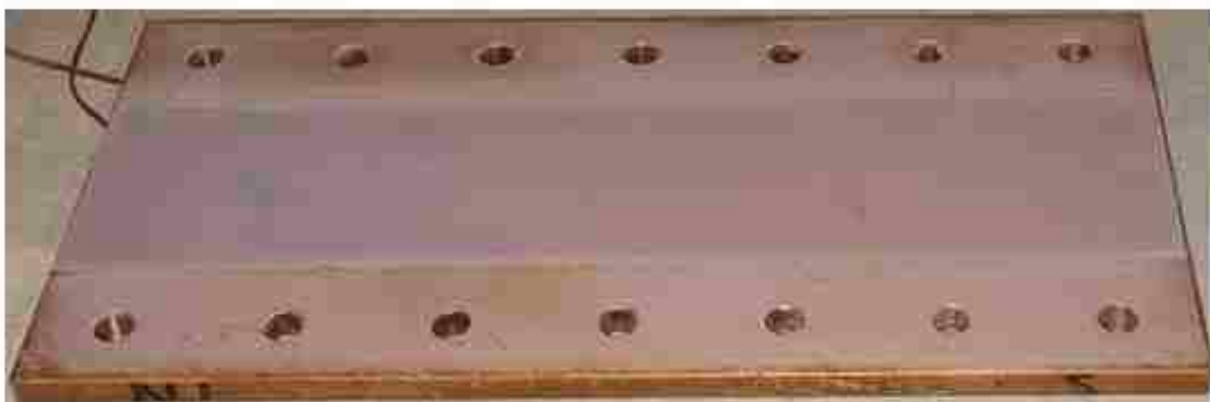
Figure 5-10: Photograph of the aerosol spray coated Rust-Oleum® NeverWet® smooth sample.
