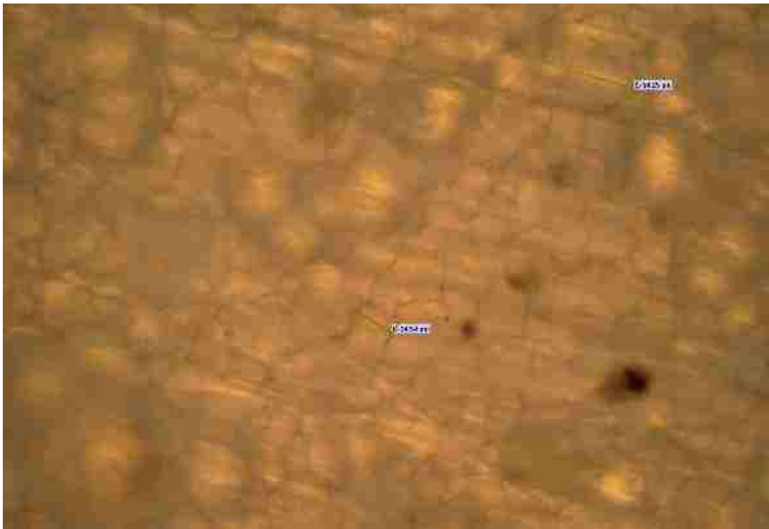
Figure 5-11: Microscope images of the Rust-Oleum® NeverWet® coating on the smooth surface copper sample at a) 10x magnification and b) 20x magnification.
