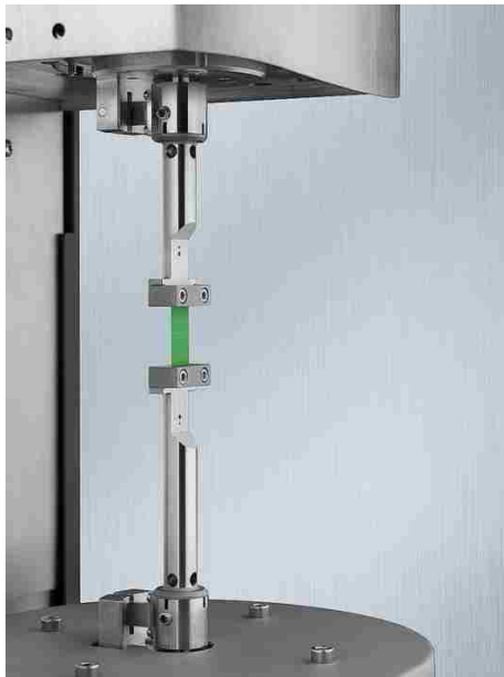
Figure 3.12: Uniaxial experimental setup on the RSA-G2 solids analyzer.
