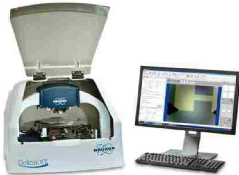
Figure 6: Image of the DektakXT machine used to take surface thickness measurements of the substrates for this experiment (Bruker, 2016).
