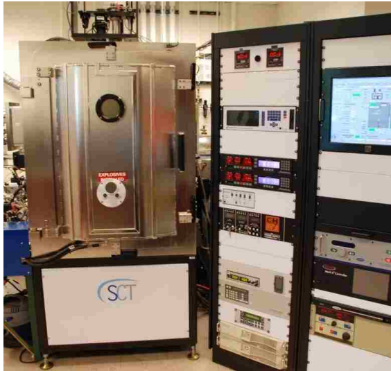
Figure 3: Custom deposition chamber used to deposit HNAB onto tantalum for this experiment, it is located at Sandia National Laboratories (Knepper, 2014).
