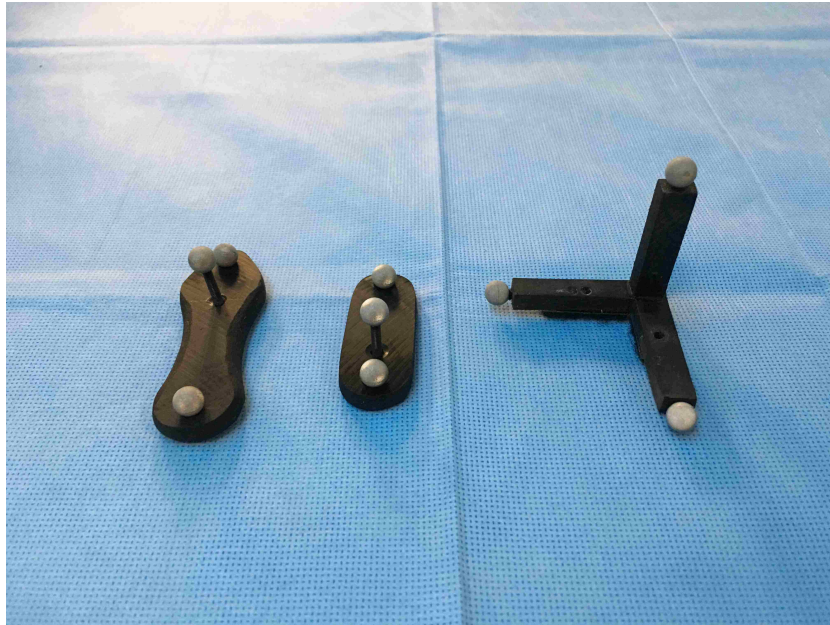
Figure 3.14: Rigid Body Markers. From left to right (Tibia, Femur, Origin)
