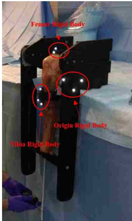
Figure 3.15: Rigid Body Marker attached during data acquisition for Varus Angulation at 90^\circ of flexion. The positions of the Tibia, Origin, and Femur rigid body sets are highlighted.
