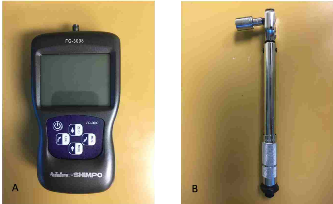
Figure 3.7: (A) Nidec-SHIMPO FG-3008 Force Gauge. (B) 5 Nm Torque Wrench.
