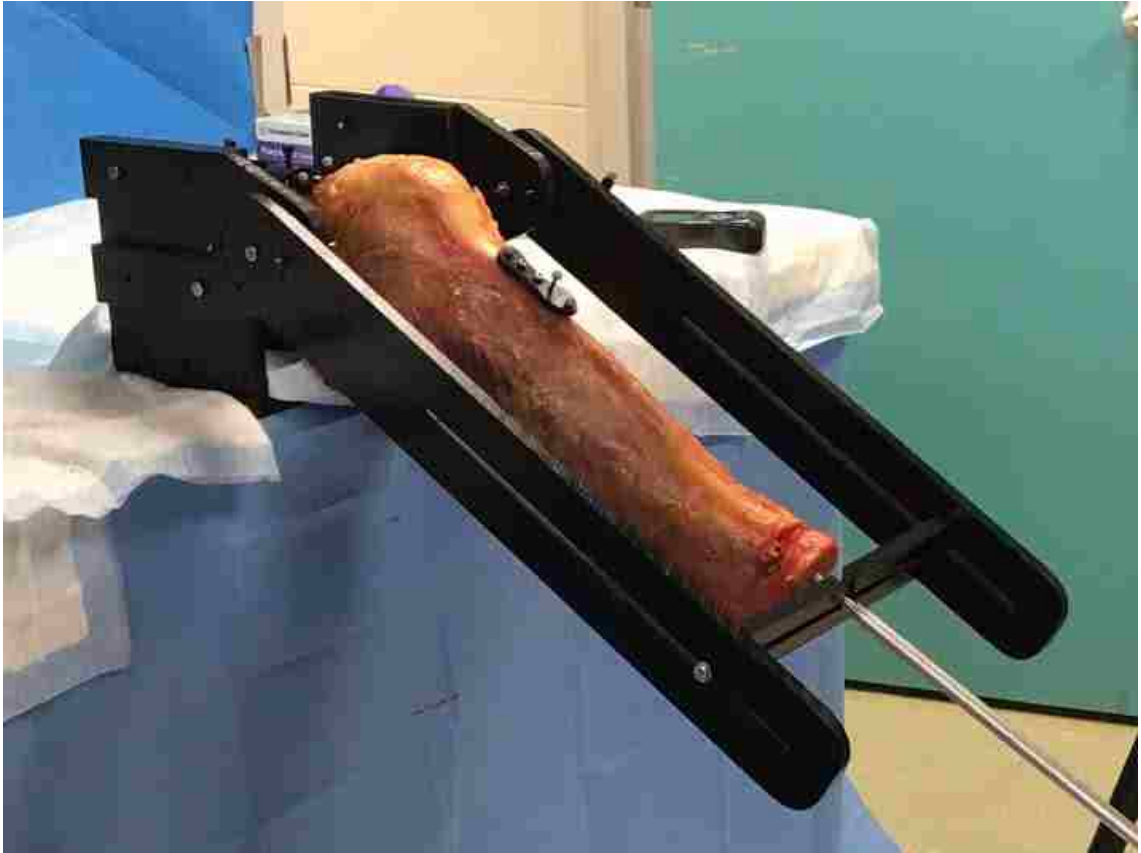
Figure 3.18: Side view of the prepared specimen mounted in the testing fixture at 30° of flexion.
