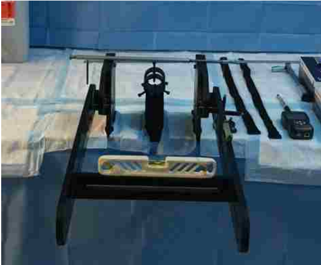
Figure 3.1: Completed Posterolateral Corner testing fixture.
