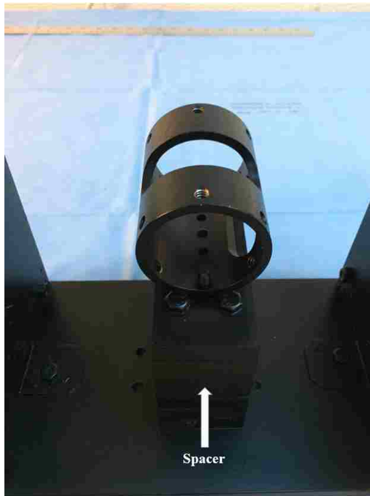
Figure 3.6: Vise and Spacer mounted on the Base Plate
