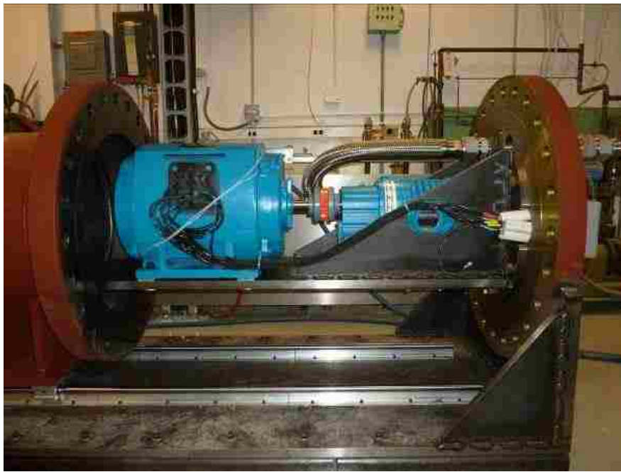
Figure 1.3: Photograph of the Roots Blower (Left) and Motor (Right) Mounted to a Plate Cantilevered of the End of the Pressure Vessel Flange Plate. The Other End of the Pressure Vessel Slides Back and Forth Over the Motor and Blower on Rails Bolted to the Skid Plate
