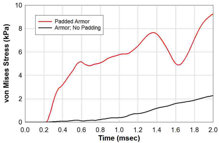
Figure 12: Heart pressure (top) and von Mises Stress (bottom) histories with the comparison between torso protected with chest armor backed by foam padding versus armor without padding.
