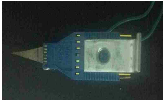
Figure 12. Finger in electroded holder (Top View)
