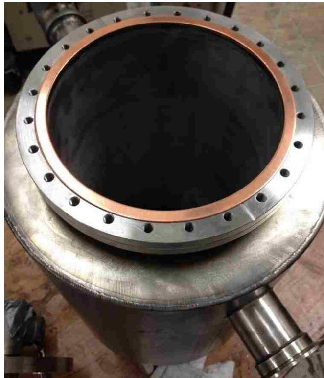
Figure 31: (Top) 32 Pin Connectors for Electrical Feedthrough (bottom) Copper Gasket for CF Flange
