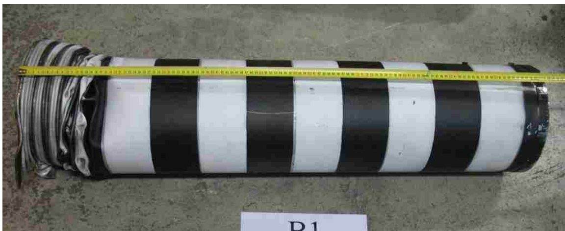
Figure 5.24: Deformed hollow missile from VTT experiment
