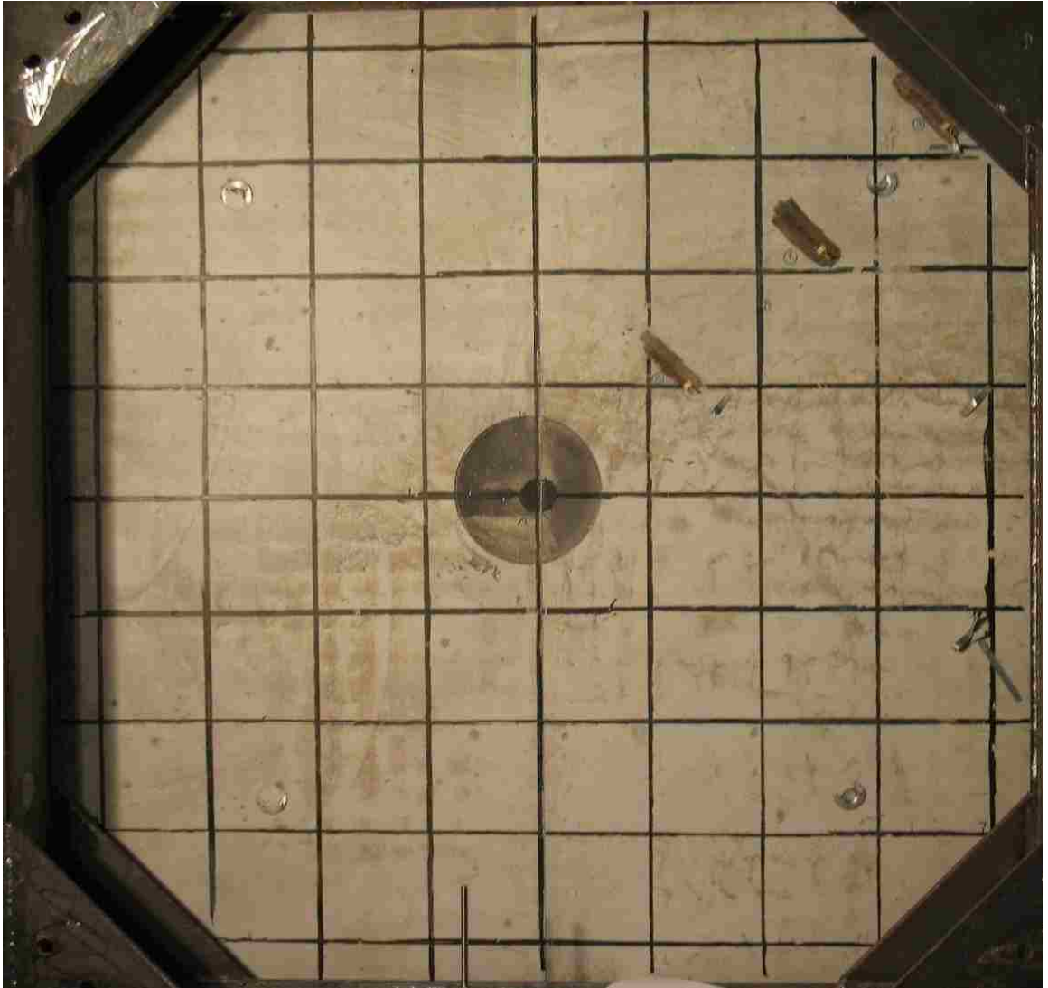
Figure 5.27: Concrete damage on front surface of VTT experiment
