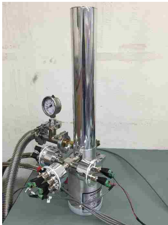
Figure 16. Advanced research system (ARS) Cryostat or cryogenic vacuum chamber.
