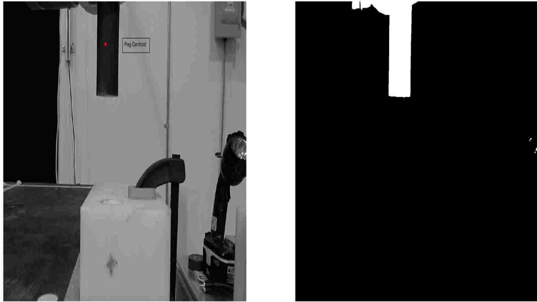
(a) Image with Peg and Centroid detected (b) Binary image of peg detected
