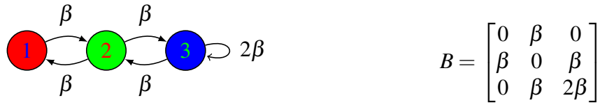
Figure 6.7: Quotient graph of the 9 Nodes Network 6.6. Colors distinguish the orbits of the automorphism group. The matrix B on the right describes the connectivity of the network.
