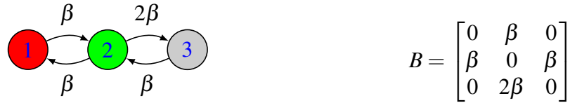
Figure 6.3: Quotient graph of the 5 Nodes Network 6.2. Colors distinguish the orbits of the automorphism group. The matrix B on the right describes the quotient network.
