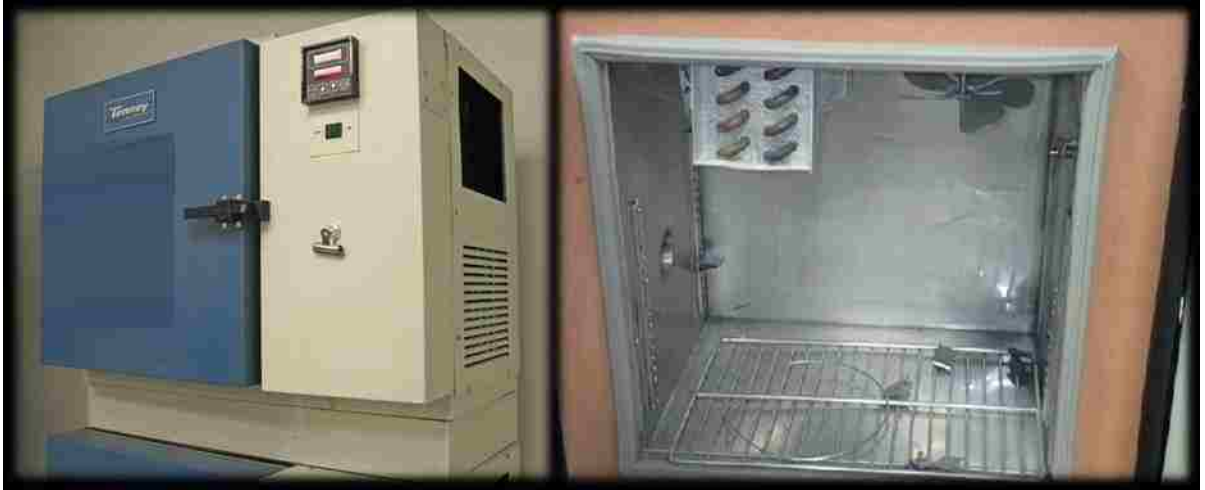
Figure 19: Temperature cycling chamber. TSJR by Tenny Environment.
