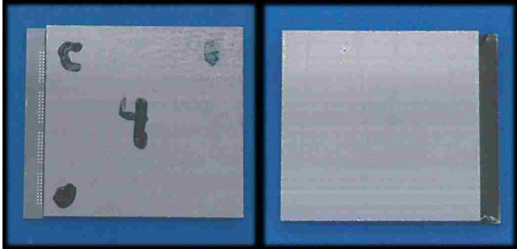
Figure 12: Typical bonded UBM sample, (Left) Top view. (Right) Bottom view.
