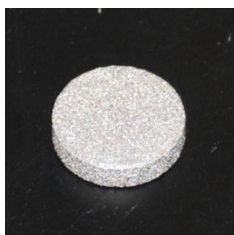
Figure 3- 3: Porous filter. The filter is 12.7 mm is diameter and is made of stainless steel. Pore size is 20 \mu\text{m} and was 40% porosity.
