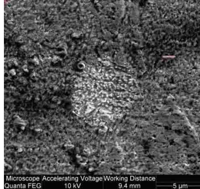
Figure 2.3: Single Shot Feature on Cu at 0.02 \mu\text{J}/\text{cm}^2
