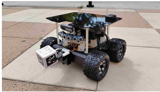
Figure 5.14: The physical robot on which components of the CPFA have been implemented
