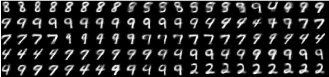
Figure 3.12: Slow sampling version of the chains model trained on the MNIST dataset with a chain length of 1000. Samples show natural-looking transitions, with some jumps. It is likely that the RNN has learned how to generalize and is not simply sampling from a mixture over the training set.
