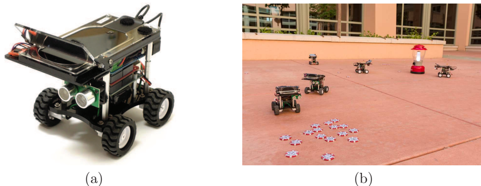
Figure 4.1: (a) An iAnt robot. (b) A swarm of iAnt robots foraging for resources around a central illuminated beacon.
