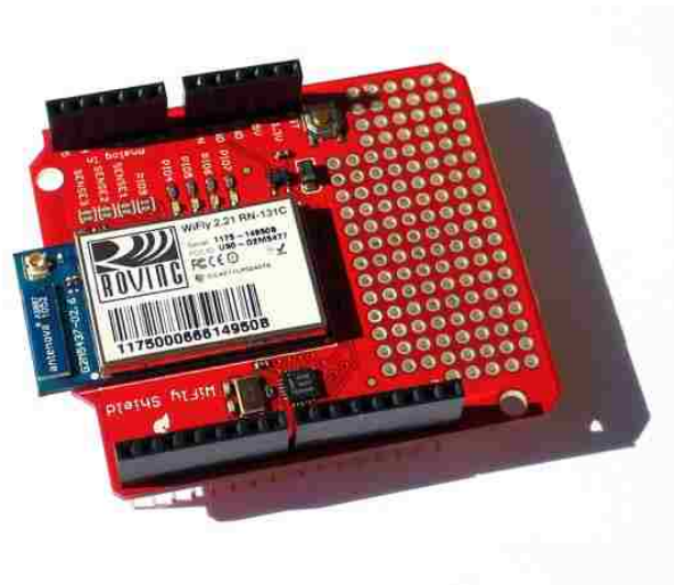
Figure 2 - The Roving Networks Wifly module on mating Arduino shield.
