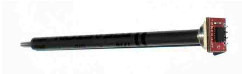
Figure 6 - HMC6352 Compass module on aluminum stalk. Threaded end replaces chassis top-plate mounting screw. Mounting plate is slip-fit in tube to allow alignment.
