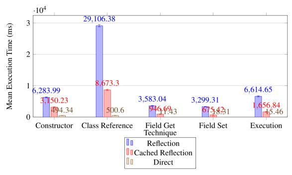
Figure 4.1: Mean execution time for 10 trials of 100,000 iterations of each sample low-level execution. Error bars indicate 1 standard deviation. The reflection based calls require a significant amount of time to execute in comparison to direct execution. Caching does reduce the time required to execute, but still is not as fast as direct execution. This data is found in tabular form in Appendix A.1.
