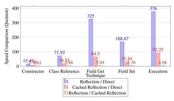
Figure 4.2: Ratio of mean execution times, comparing the 3 techniques highlighted in Figure 4.1. Although Class Reference was the slowest operation in total time, the highest percentage increase in speed is the execution and field get operations between reflection and direct execution. This data is found in tabular form in Appendix A.2
