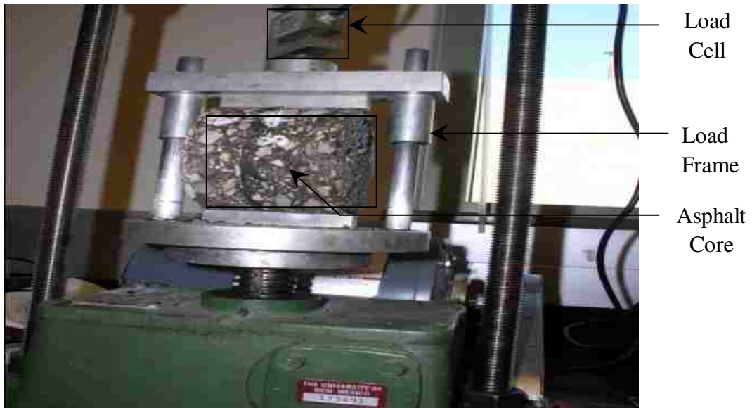
Figure 3.21 Indirect Tensile Strength Test
