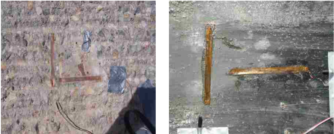
Figure 5-19 Strain gauges attached to the concrete surface and FRP strips.
