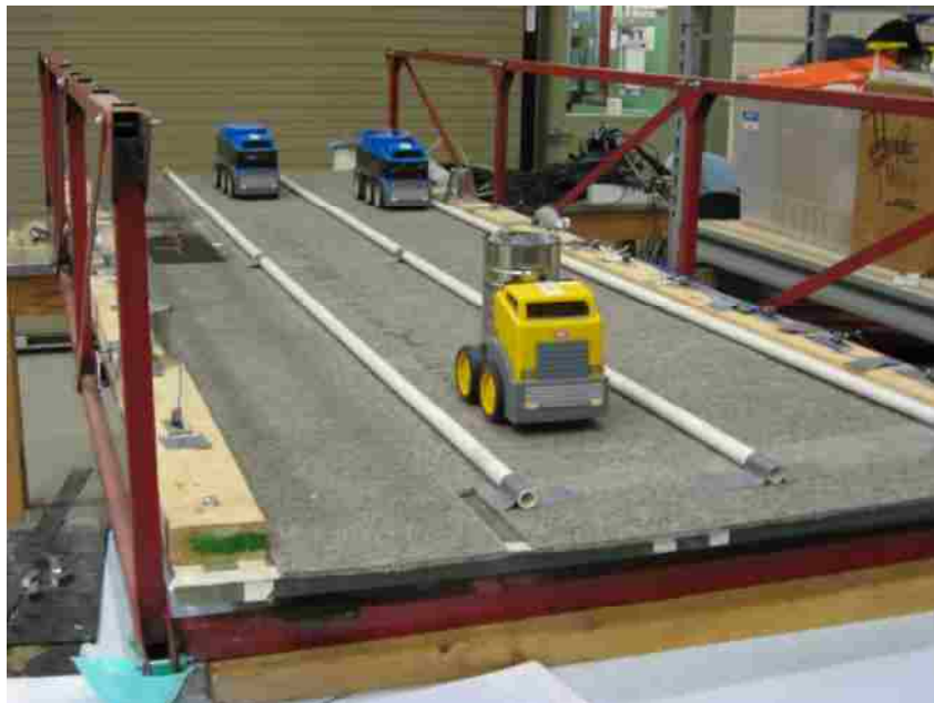
Figure 5-34 Model bridge constructed at UNM structural laboratory.
