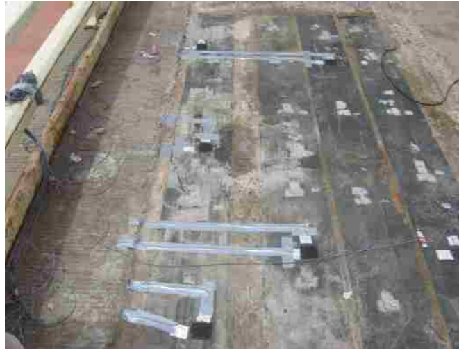
Figure 5-54 All the strain gauges after being installed on the FRP sheets and connected to the wires transmitting the strain signals to the DAQ device.
