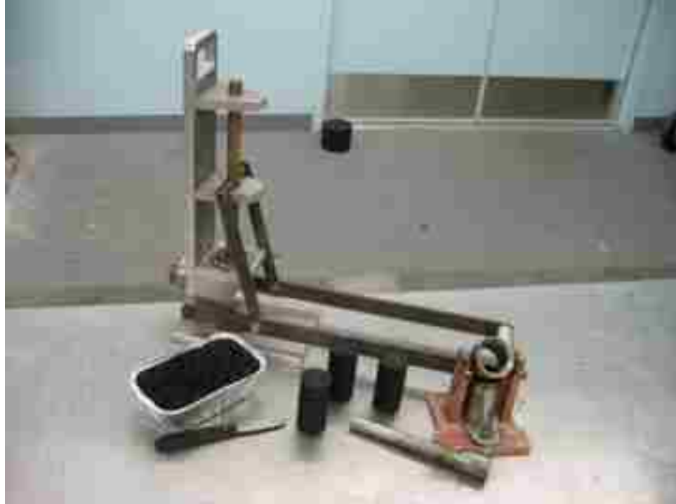
Figure 3.5 Materials for Preparation of Cylindrical Samples
