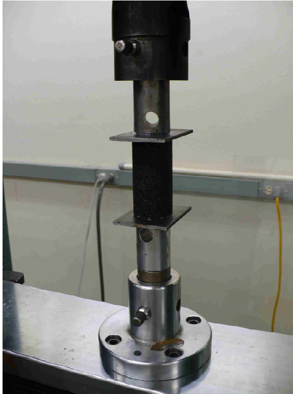
Figure 3.6 Test setup for cylindrical matrix samples
