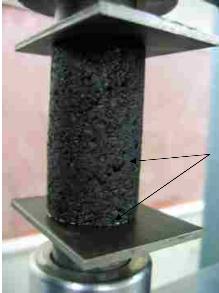
Figure 6.3 Exudation of water from matrix sample during compression
