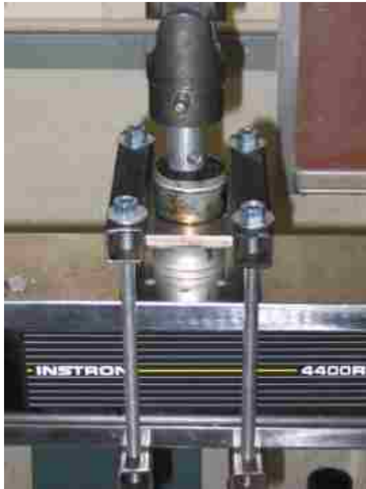
Figure 3.7 Test setup for aggregate/matrix interface in tension
