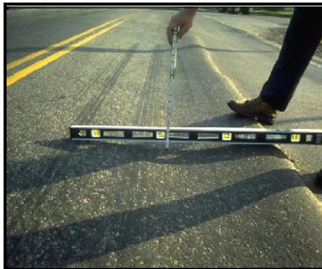
Figure 9. Measure of a rut depth on flexible asphalt pavement (From Miller & Bellinger, 2003).
