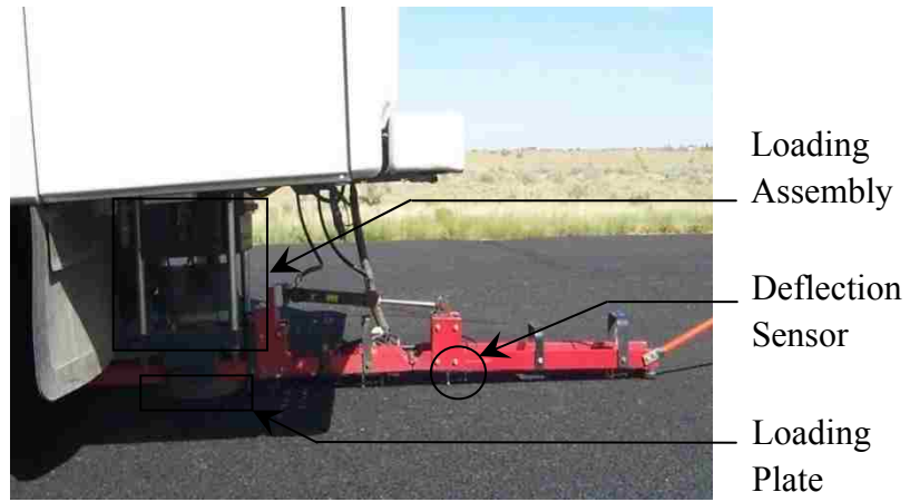
(a) FWD testing assembly (JILS FWD 20T)
