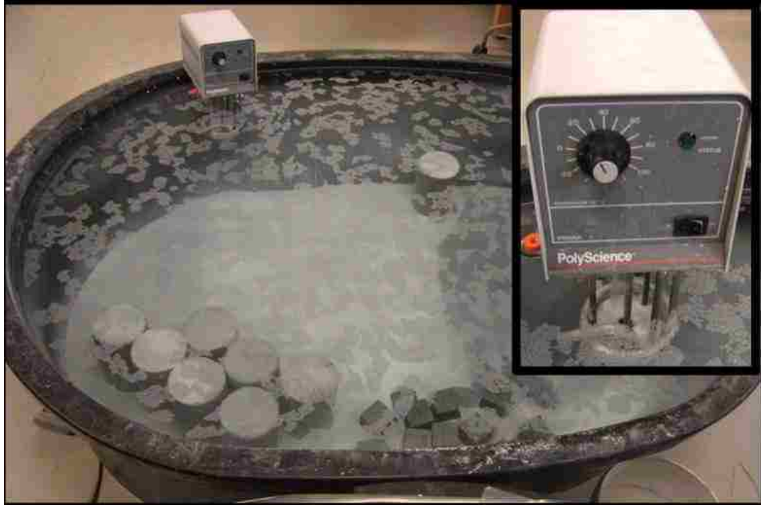
Figure 3.6. Curing of concrete specimens
