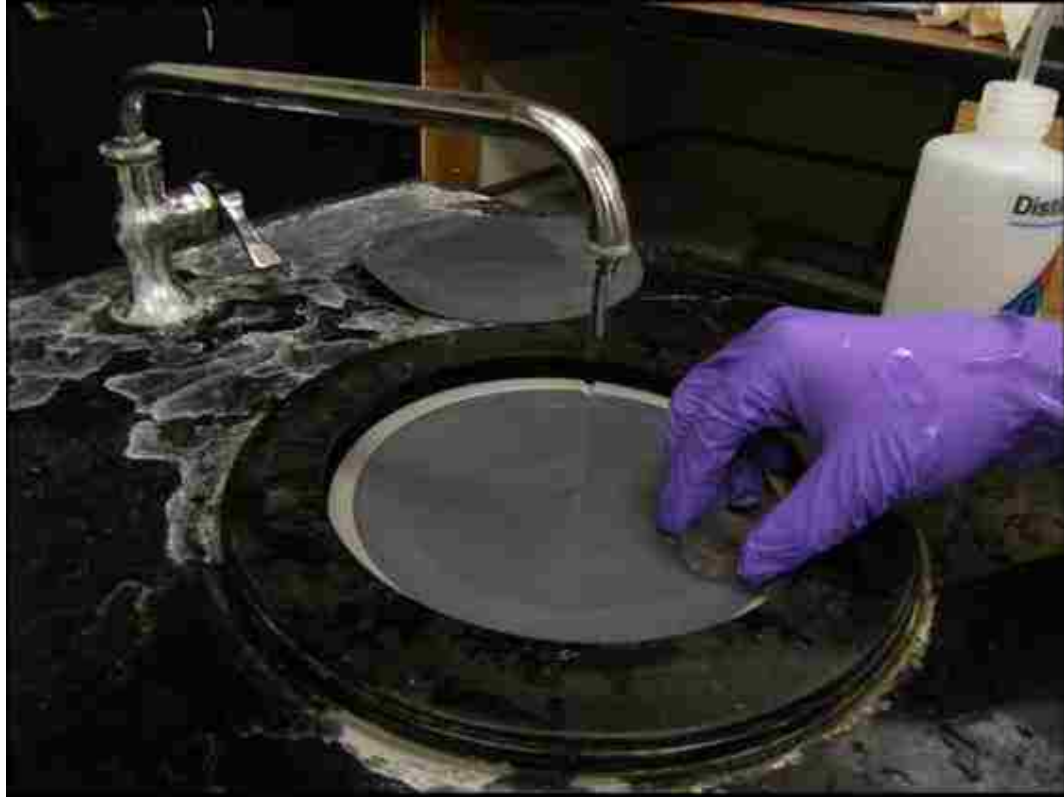
Figure 4.1. Grinding of nanoindentation sample
