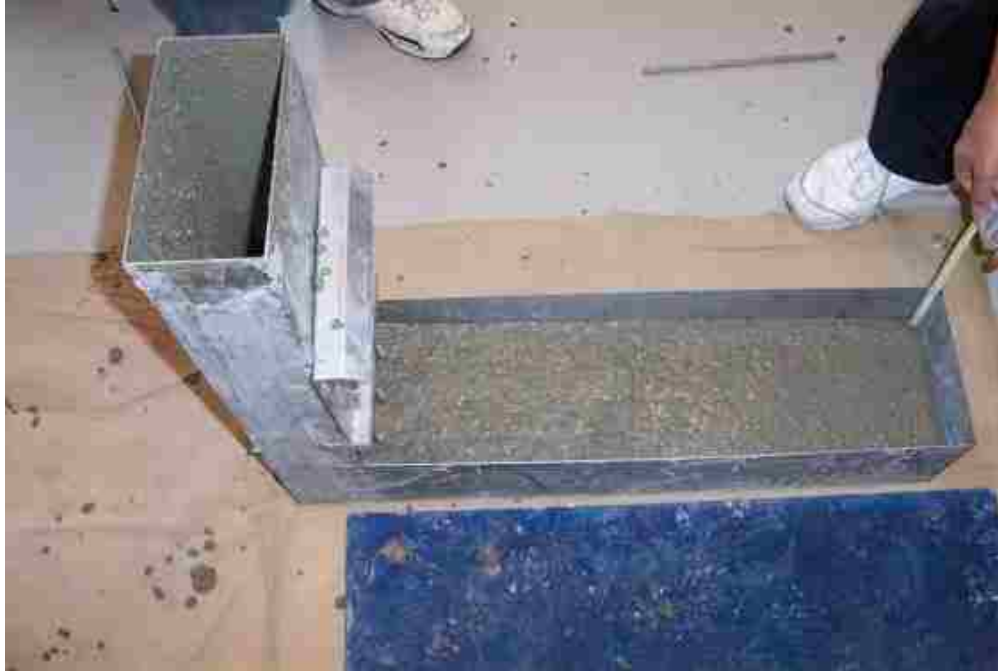
Figure 3.4. Measuring height of horizontal section of fresh SCC after L-box test
