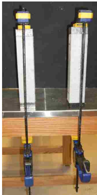
Figure 3.37. Curing of epoxy with applied pressure using c-clamps
