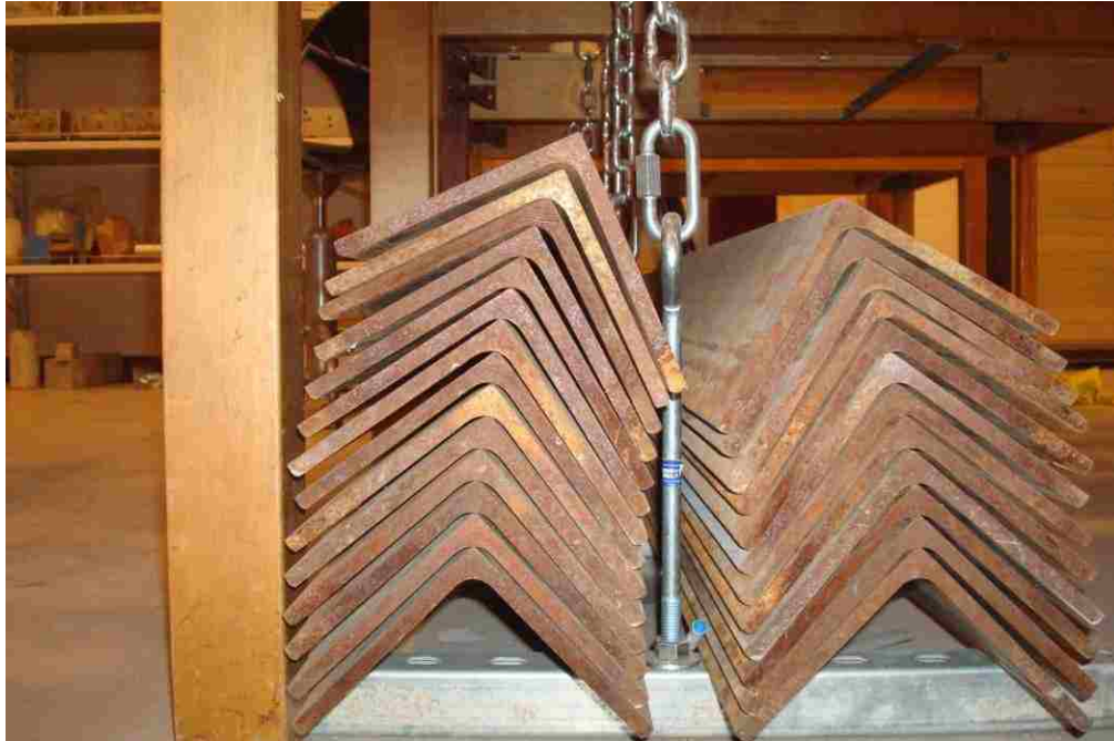
Figure 3.43. Steel chain anchored to the ground angle iron counter weights
