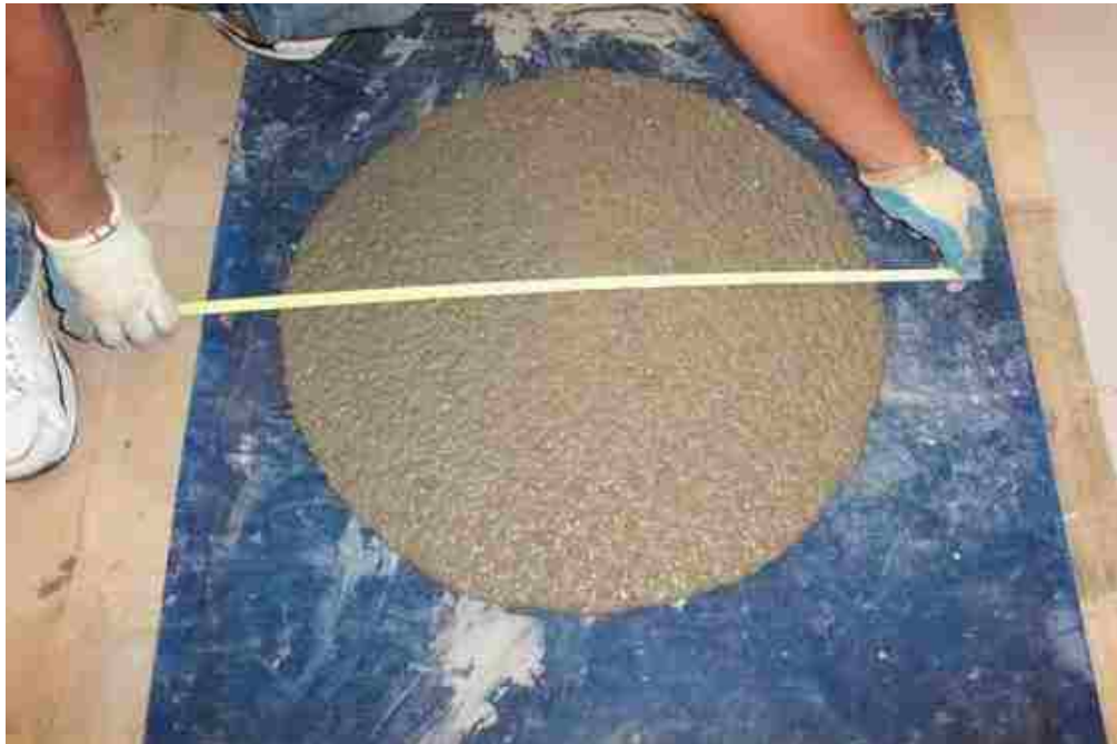
Figure 3.3. Measuring diameter of fresh SCC after slump flow test
