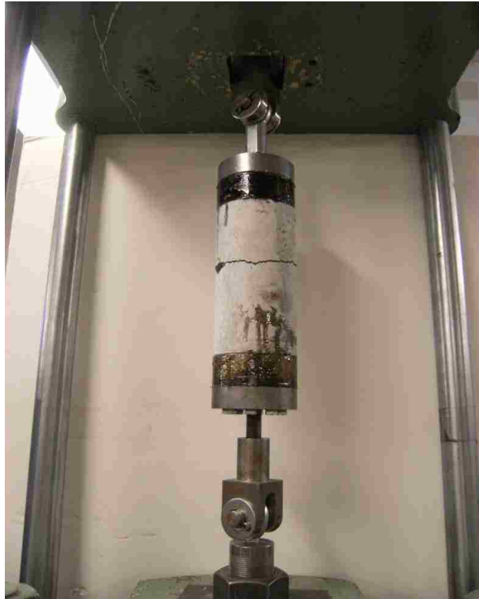
Figure 3.39. Direct tension test with fractured specimen after Kim et al.
