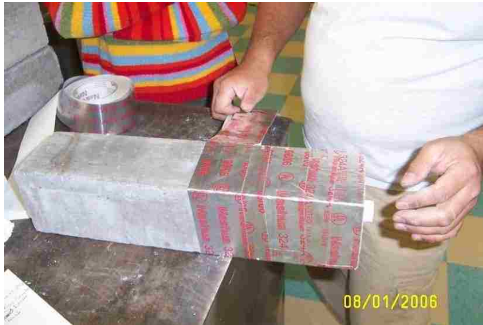
Figure 3.7. Sealing of sealed specimens with aluminium tape
