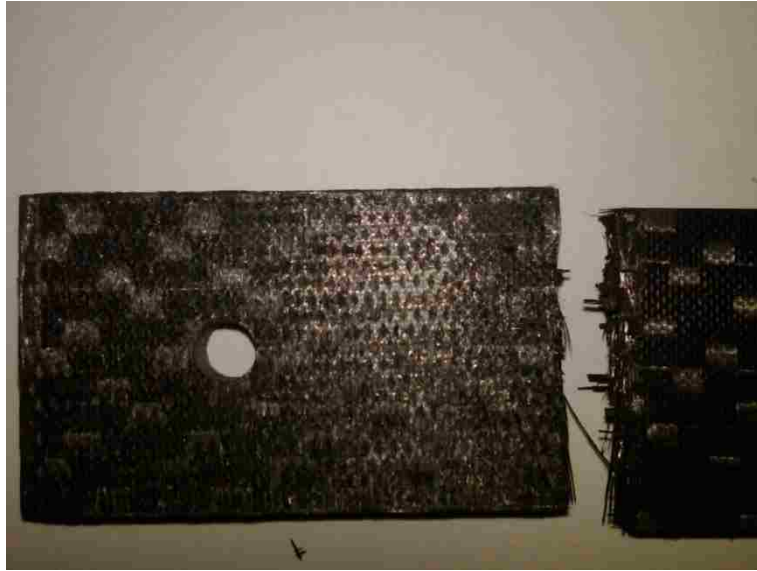
Figure 4.6: Untabbed uni-axial LAB failure in wedge grip.
