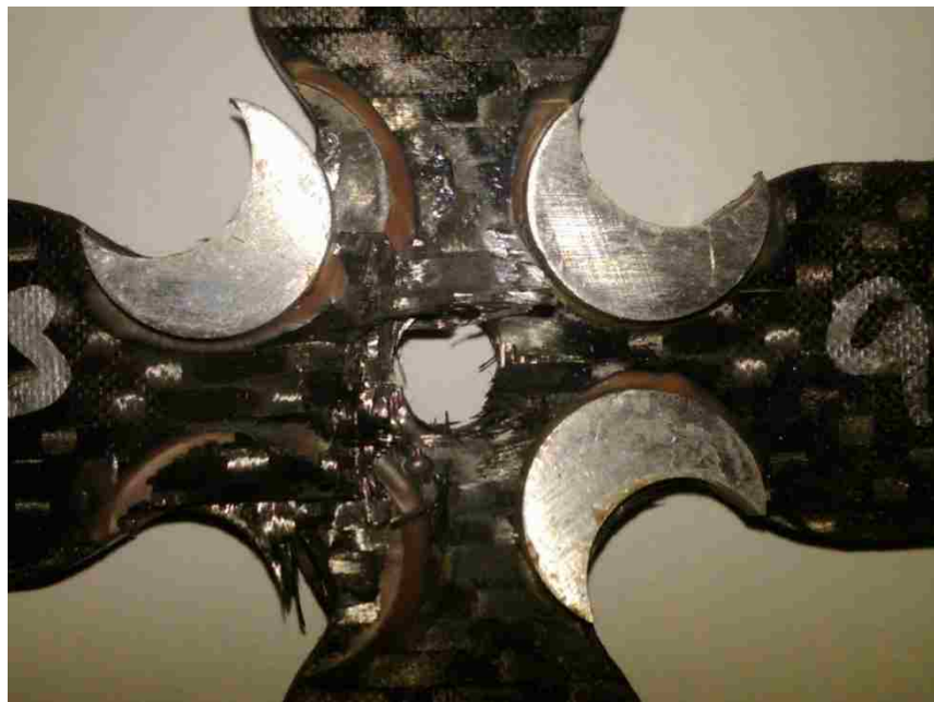
Figure 4.28: Center hole Type III shimmed specimen failure.
