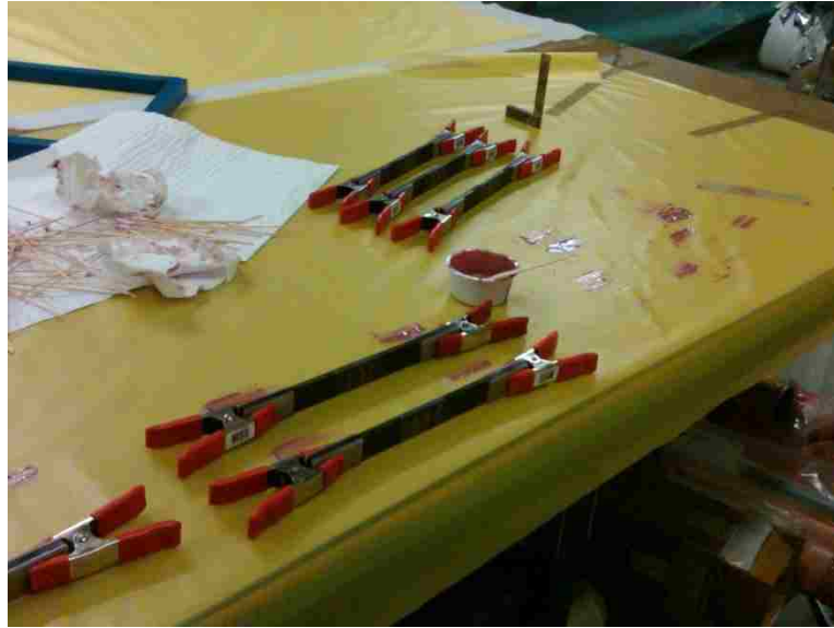
Figure 4.3: Uni-axial specimens with G10 glass tabs clamped for adhering.
