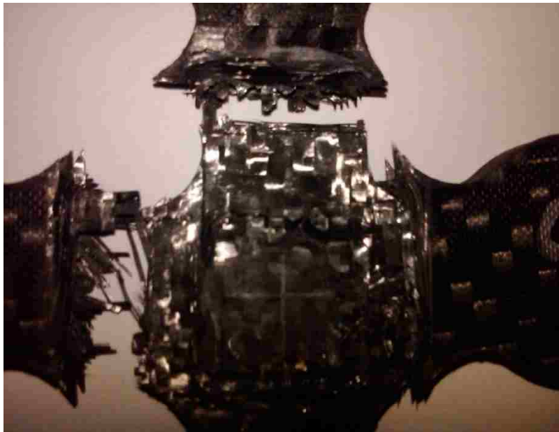
Figure 4.9: Close up of failure in the Type I control specimen.
