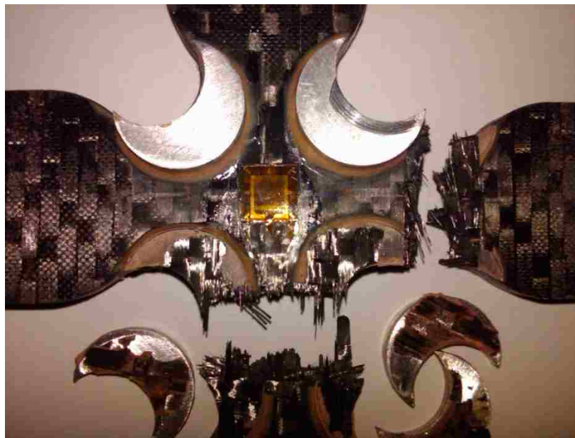
Figure 4.12: Close up photo of the Type I shimmed failure.
