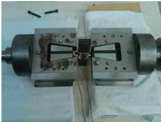
Figure 3.12: Specimen and wedge grips placed in the wedge grip arms.
