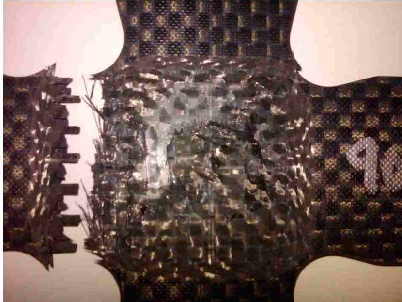
Figure 4.18: Adequate 45° failure mode for the Type II control specimen.
