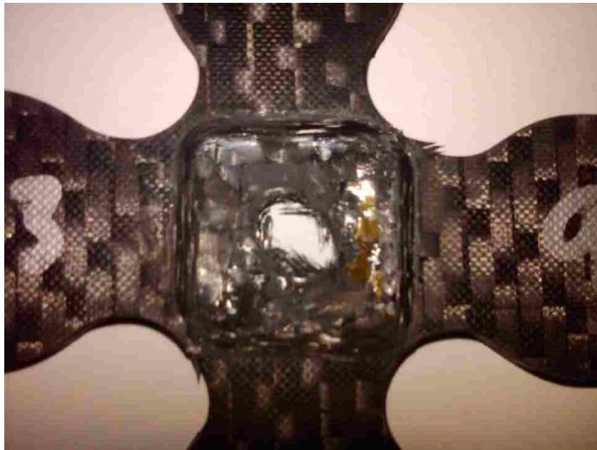
Figure 4.26: Center hole Type III control specimen failure.
