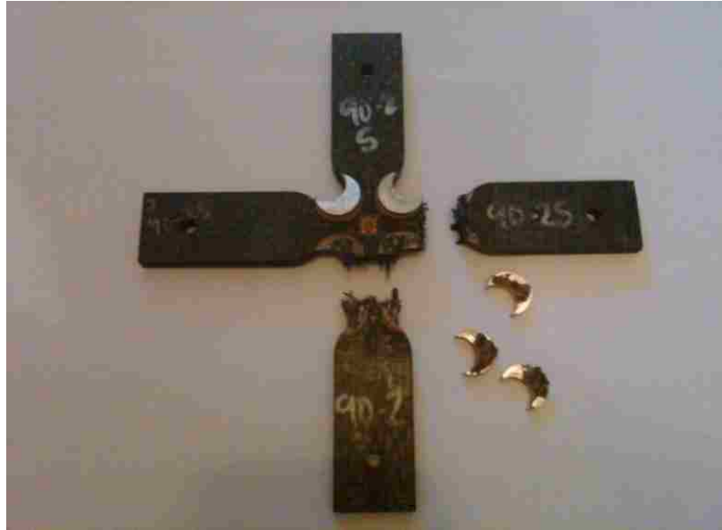
Figure 4.11: Shows a Type I shimmed bi-axial specimen failure.
