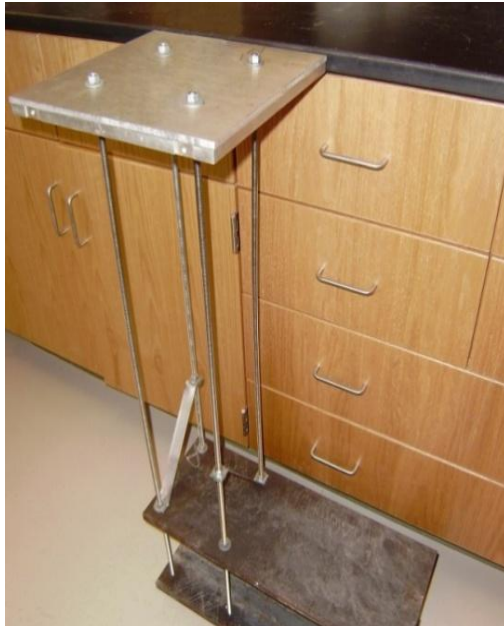
Fig. 7.4 : Vibrational System With Plates Fixed Parallel to Each Other. Assuming Small Air-Damping Effect.
