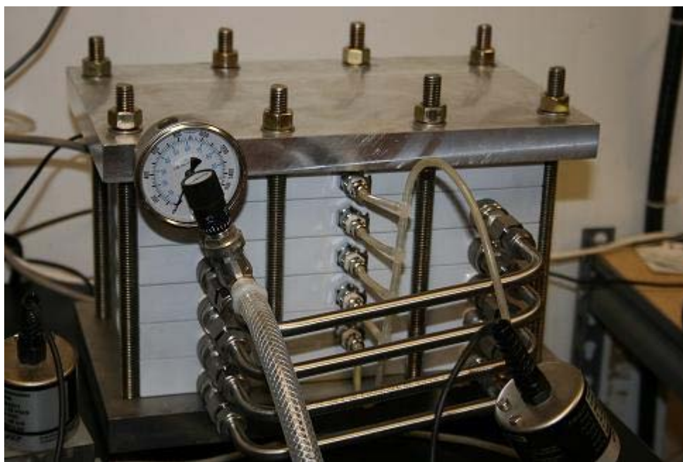
Figure 3-5: Picture of the RO Unit
