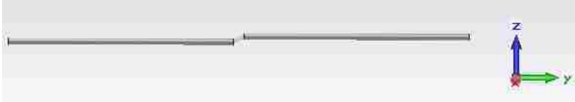
Figure 32: Half-Wave Dipole With Intentional Offset
