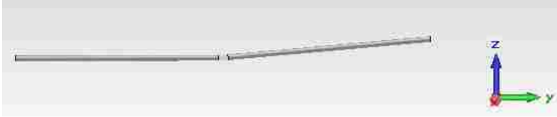
Figure 34: Half-Wave Dipole with Intentional 5° Offset.
