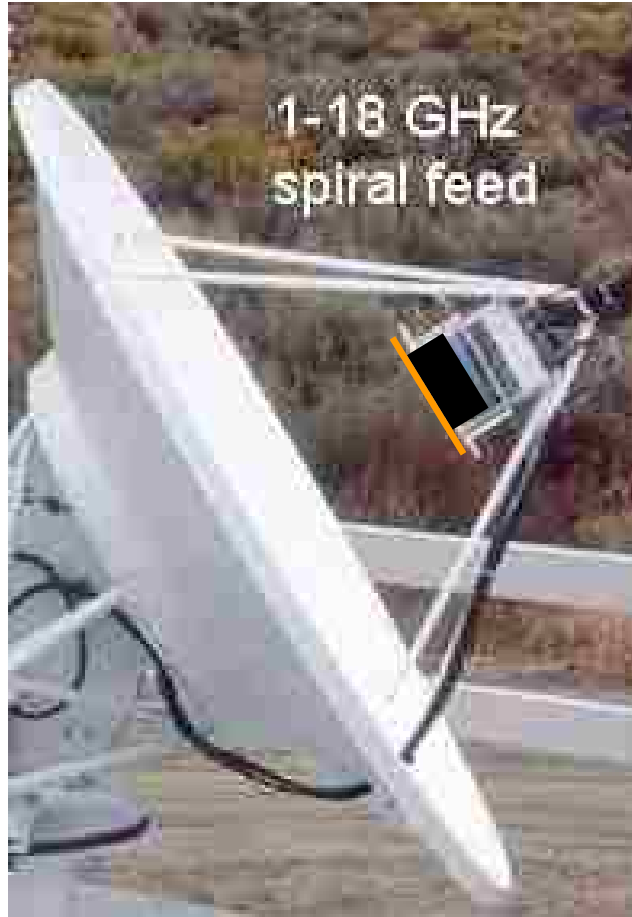
Figure 136: Mock up of diamond feed mounted in a SRBL system
