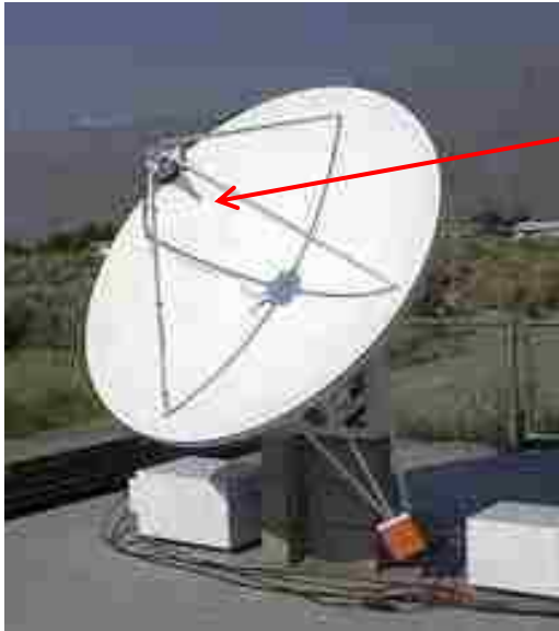
Figure 14: LPDA Feed Used in OVSA. [34]
