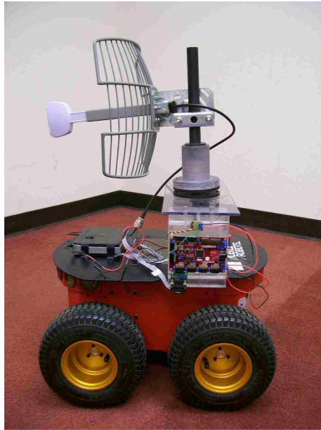
Figure 4.11: The picture of the Pioneer 3-AT robot, equipped with directional and omni-directional antennas, used for channel measurements in the indoor surveillance scenario of Fig. 4.9. Only omni-directional channel measurement were used in this example.
