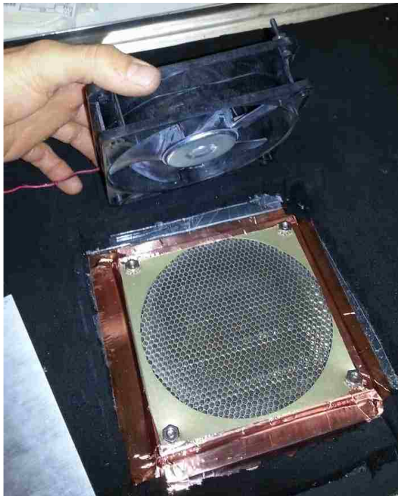
Figure 4.4: Vent fan being affixed to RFI Honeycomb, attached to enclosure by copper tape.
