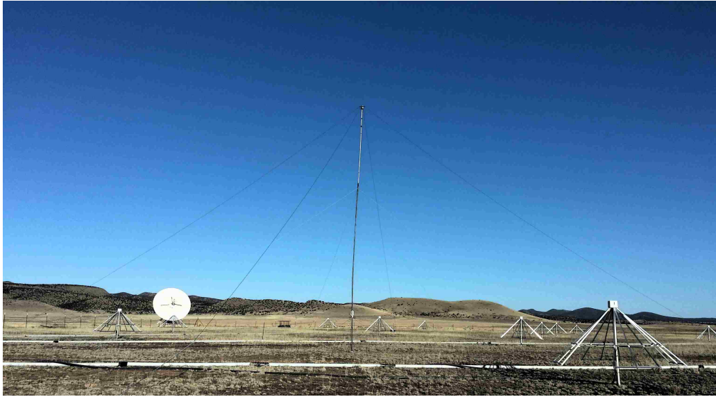
Figure 2.1: Left background: The 25-meter VLA dish antenna. Center: 35' high, 95' wide HF-optimized antenna. Right: LWA Antenna.
