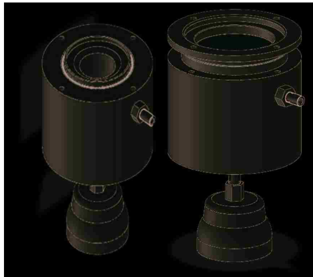
(a) Fixture 1, which used screws to hold down the B1 and seal the fluid in place.
