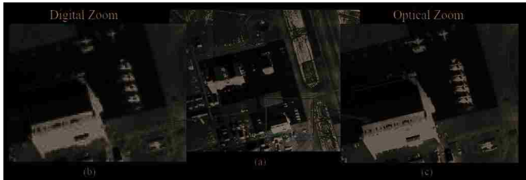
Figure 1.2: (a) Airfield image.(b)Digital zoom, no resolution improvements, pixelated image.(c) Optical zoom showing and increase in magnification and resolution
