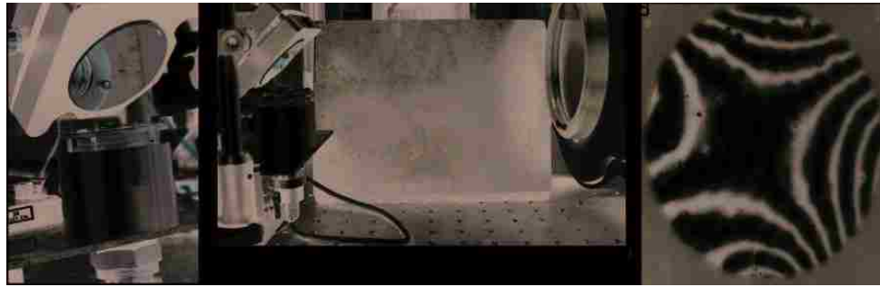
Figure 3.14: (Left) Shows the B1 hold by 4 screws and the washer, with incident laser from the Zygo interferometer. (Middle) Setup in front of Zygo. (Right) Analog image of the full aperture of the membrane obtained from the Zygo. Astigmatisms can be clearly seen on the image, depending on how the screws were modified the magnitude and direction of it could be alter.
