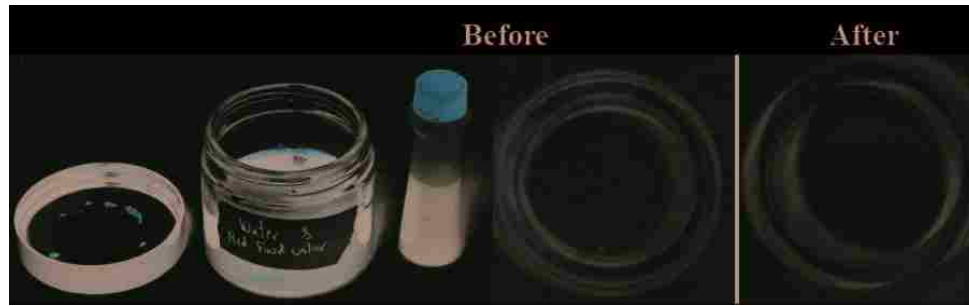
Figure 2.21: (Left) Red dye solution in which bond with membrane was submerged showing the marks of dye on the bonding area. (Right) Bond with membrane under new procedure after been submerged in the same red dye solution. No dye was seen on the bonding area.
