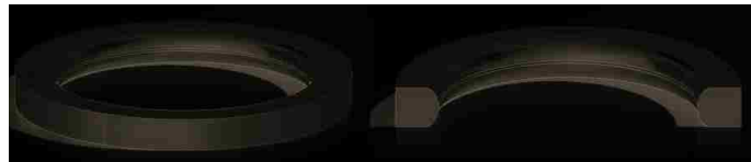
Figure 2.27: Conceptual ring with radial profile in the ID for membrane deflection.
