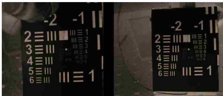
Figure 2.13: Thiol-ene membrane and PDMS in front of an Air Force resolution target chart
