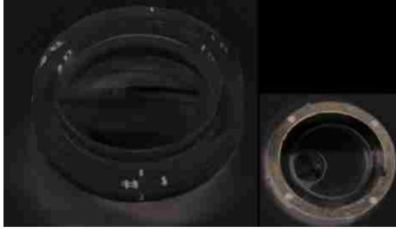
Figure 2.6: Air bubble inside a strong negative lenscore
